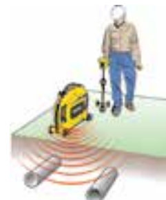
Induce a signal to locate utilities.
