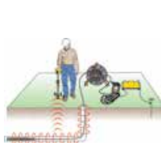
Find plastic pipe with integral line trace.
