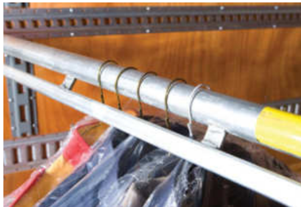
Bar rotates to lock garments in place.
