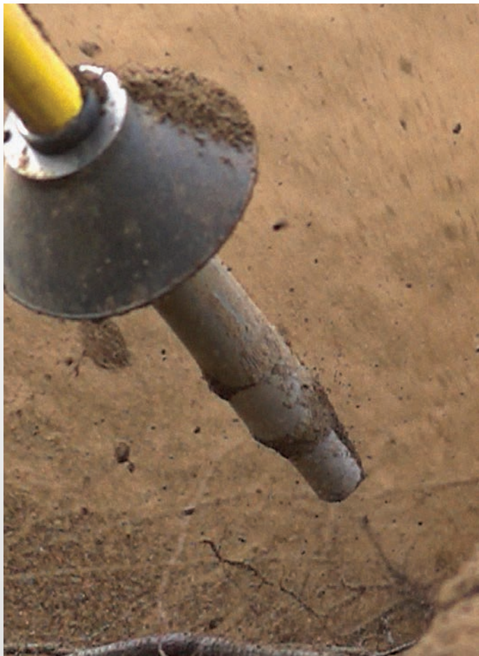
Unfocused air flow from improperly designed nozzle.
